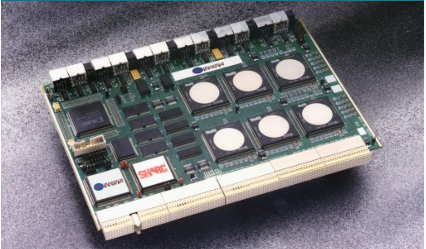
**A**imed at high performance, floating-point DSP applications, the ASP-S60 merges the power of six SHARC DSPs with the speed of CompactPCI and front end processing of a Xilinx XC4028EX FPGA. The result is a highly flexible processing engine ideally suited to professional audio, sonar and telecommunications applications.
