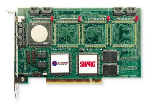
he ASP-P14 is a minimum cost SHARC DSP PCI card supporting a single Analog Devices ADSP-2106x processor with up to 12Mbytes DRAM and 512kbytes of FLASH memory. For the highest levels of PCI throughput, the ASP-P14 also provides a PCI interface which can sustain data transfer rates of over 120Mbytes/sec. This is complemented by a hardware data type conversion to assist the exchange of data between PCI and SHARC environments.
