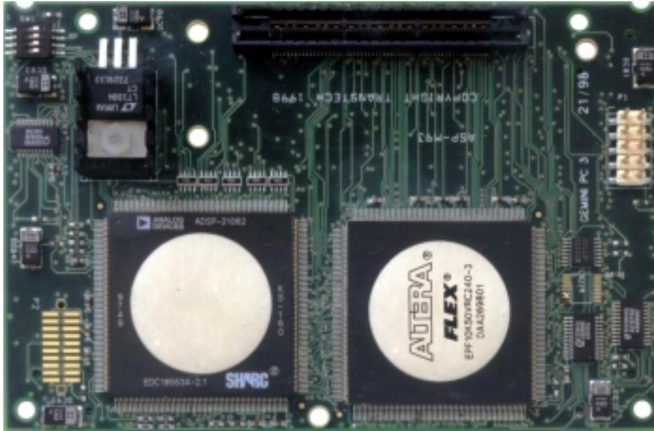
**T**he ASP-M93 provides high speed digital I/O to SHARC DSP based boards at up to 160Mbytes/sec via an FPGA and ADSP-2106x processor. The ASP-M93 is aimed at applications for including radar, sonar and real-time imaging processing.
