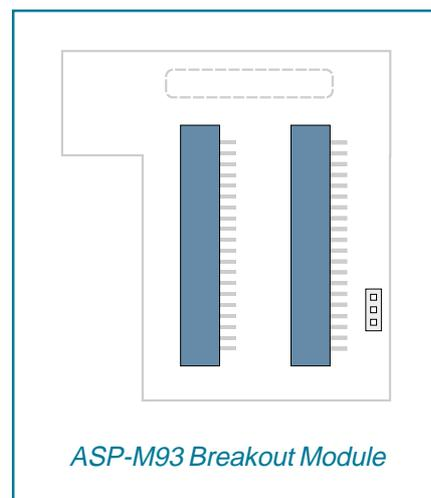
access to 50 I/O signals through two 40-way IDC headers.
